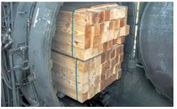
pressure treatment. PET strapping has the strength of steel strapping but unlike steel, it has elastic properties to stretch and hold the expanding package secure without cutting into and deforming the wood. Straps stay tight and absorb impacts without breaking.
