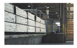
Polyester (PET) it the strapping of choice Here, the lumber emerges from for pressure treated wood thanks to its elongation and recovery characteristics. Loads of lumber are unitized before treatment. The PET strap does not corrode from the treatment chemicals unlike steel strapping that can rust and stain the wood.
