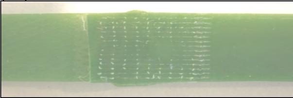
**NO – seal strength insufficient**
