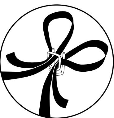
How to Thread Cord Strapping onto Metal Buckles
