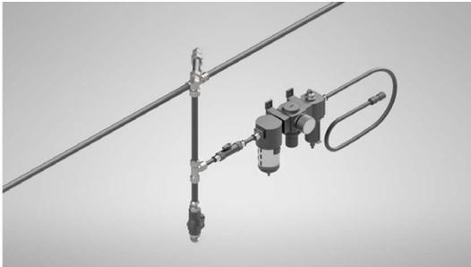
There are TWO important functions, pressure and volume. Without the proper volume as well as pressure, the tool will not perform or function properly. The air line should be constructed according to this diagram and drained daily.
