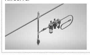
There are TWO important functions, pressure and volume. Without the proper volume as well as pressure, the tool will not perform or function properly. The air line should be constructed according to this diagram and drained daily.
